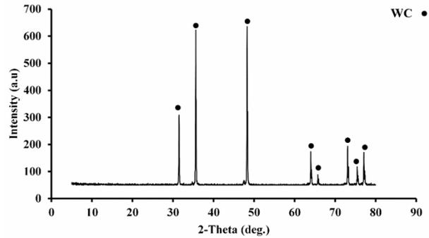
Fig. 1. XRD pattern of powder of tungsten carbide
