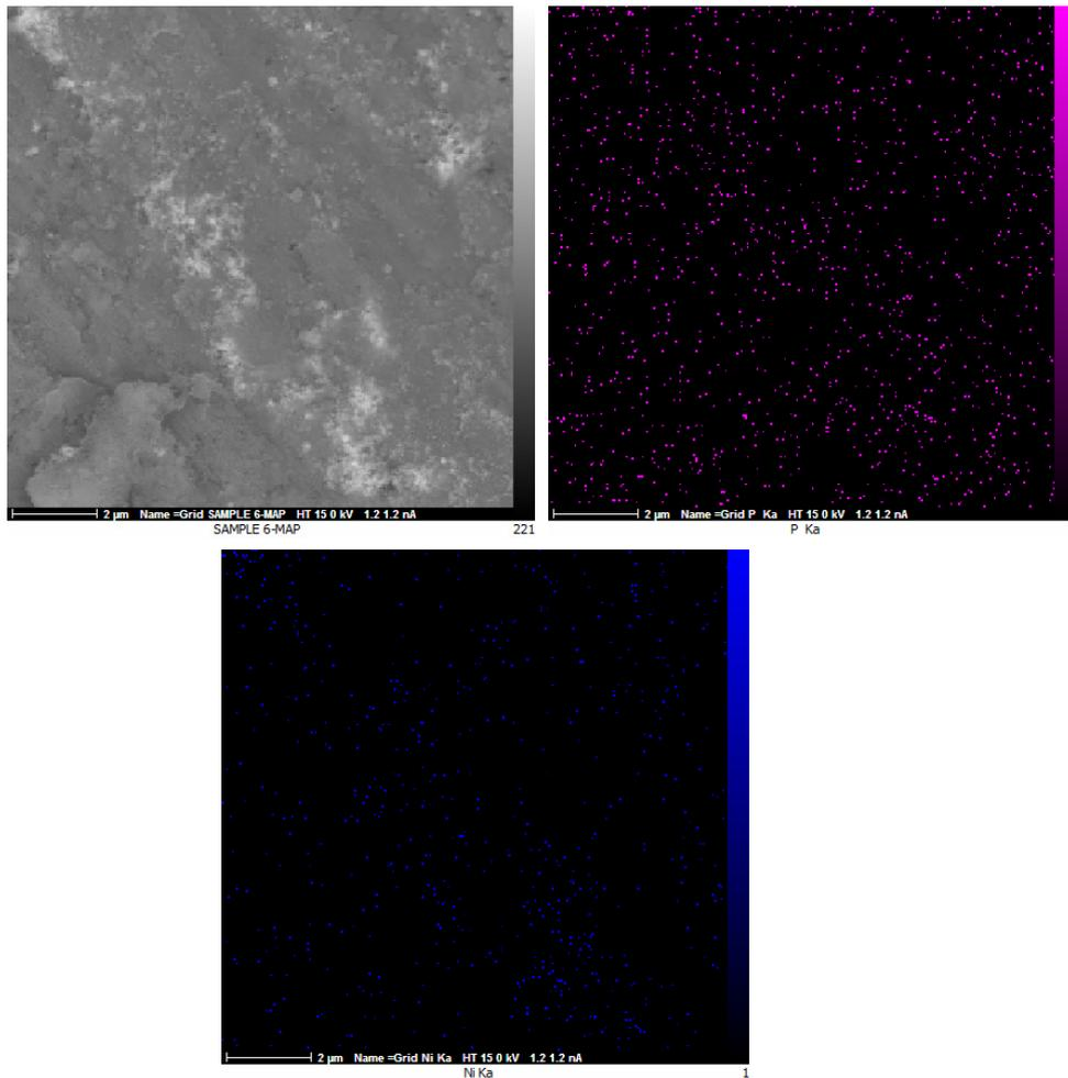
Fig. 2. MAP analysis of Ni-P distribution on alumina nanotube in 10 minutes, violet is P and blue is Nickel particles
