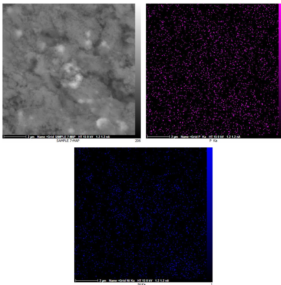
Fig. 1. MAP analysis of Ni-P distribution on alumina nanotube in 20 minutes, violet is P and blue is Nickel particles
