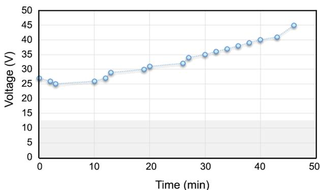
Fig. 2. potential rate profile for anodizing of Aluminum alloy in oxalic acid additive
