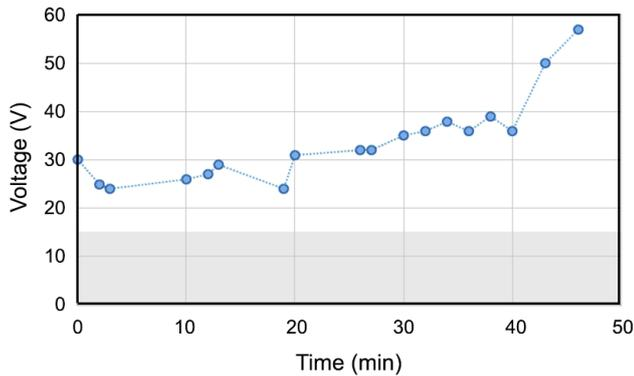
Fig. 5. potential rate profile for anodizing of Aluminum alloy in Salicylic acid additive
