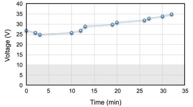
Fig. 3. potential rate profile for anodizing of Aluminum alloy in etidronic acid additive
