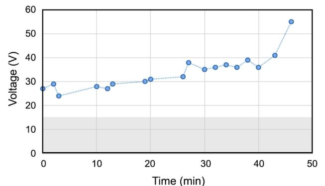
Fig. 4. potential rate profile for anodizing of Aluminum alloy in selenic acid additive
