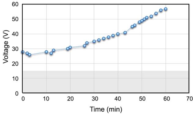
Fig. 1. potential rate profile for anodizing of Aluminum alloy in tartaric acid additive
