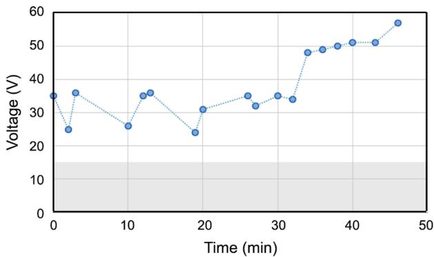
Fig. 6. potential rate profile for anodizing of Aluminum alloy in citric acid additive
