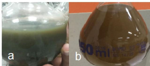
Fig. 1. a) Aqueous solution of plant seeds extract. b) Aqueous solution of FeNPs in plant seeds extract.
