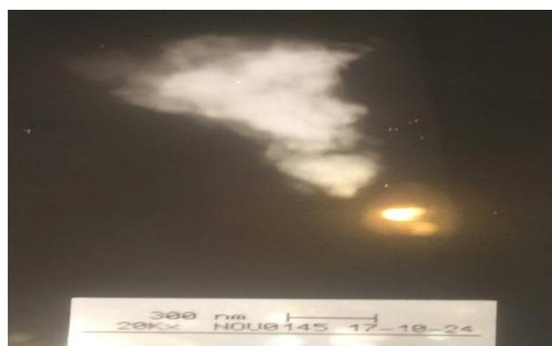
Fig. 2. TEM image of FeNPs synthesized by aqueous extract of *Carum carvi L.*
