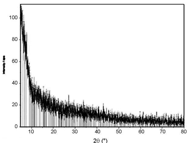
Fig. 5. XRD spectra of chitosan-coated FeNPs
