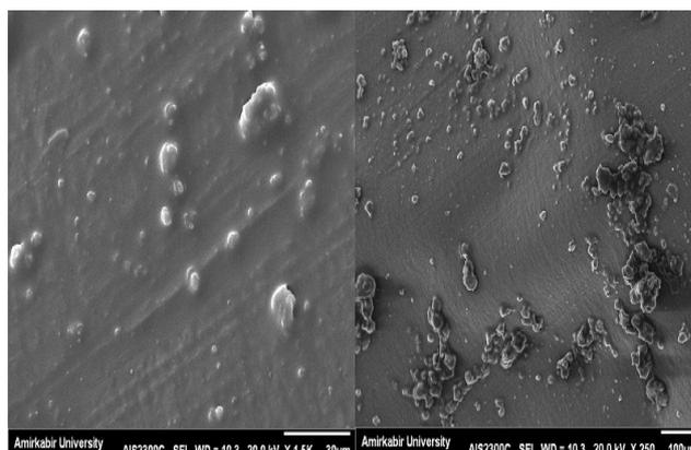
Fig. 3. SEM images of FeNPs synthesized by aqueous extract of *Carum carvi L.*
