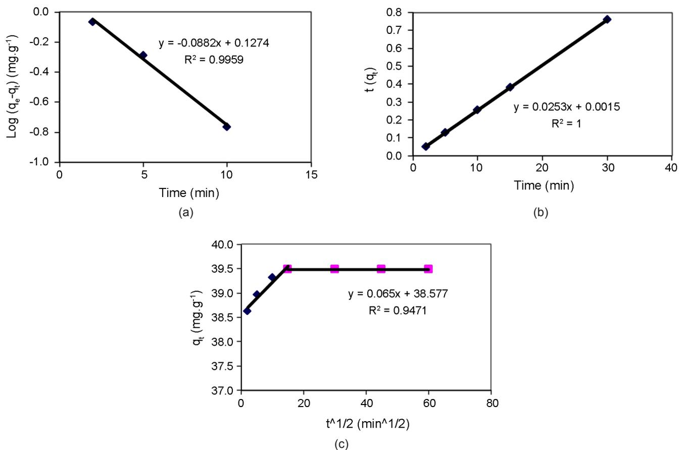
Fig. 8. Adsorption kinetics of doxorubicin on 0.005 g FeNPs at temperature of 298 K: (a) pseudo-first-order; (b) pseudo-second-order; (c) and intra-particle diffusion models.
