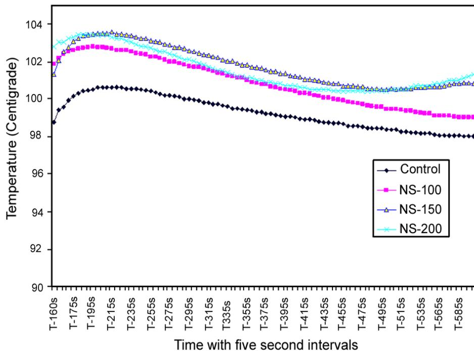
**Figure 4:** Temperature at the core section of the medium density fiberboard mat after the third minute of hot pressing with five second intervals (NS= nanosilver content mL/kg).
