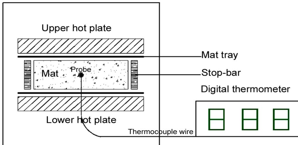
Figure 2: Temperature measurement using a digital thermometer with its sensor probe inserted into the core section of the composite board mat.
