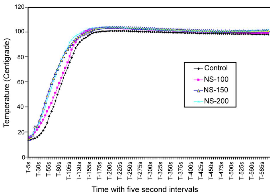
**Figure 3:** Temperature at the core section of the medium-density fiberboard mat with five-second intervals (NS= nanosilver content mL/kg).
