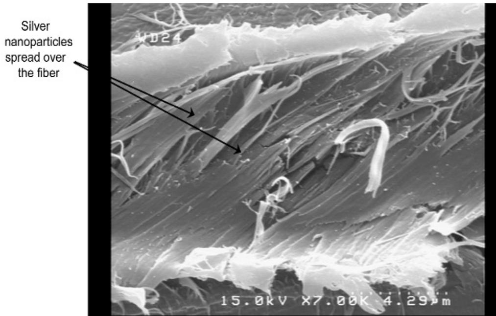
Figure 1: SEM micrograph showing nanosilver scattered all over the fibers.
