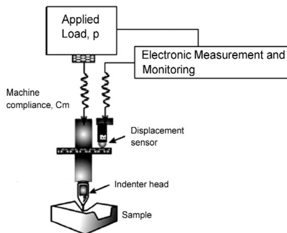
**Figure 1:** Different parts of a typical indentation instrument [2].
