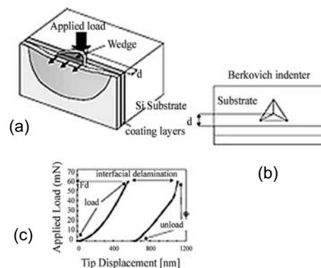
**Figure 4:** (a) A schematic presentation of cross-sectional nanoindentation (CSN) technique in multi-layer thin films, (b) Berkovich indenter with respect to thin film interface, (c) a sudden jump in Load-displacement curve corresponding to thin film delamination [42].
