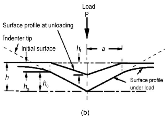
**Figure 2:** (a) A typical nanoindentation : load and unloading -displacement curve and schematic loading cycle in CSM technique (b) schematic deformation pattern of substrate surface with an elastic-plastic behavior after indentation test [1, 14].
