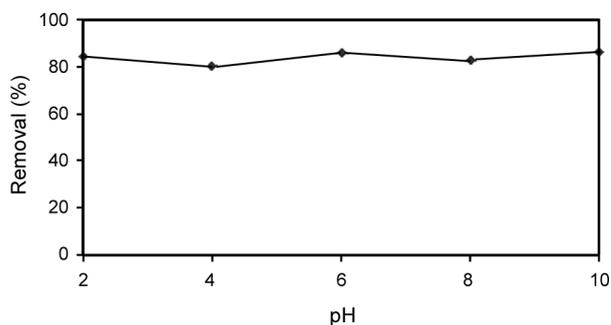
**Figure 2:** Effect of pH on adsorption of CNB onto MWCNTs.  $[CNB]_0=16$  mg/L;  $[MWCNTs]_0=0.1$  g/250mL; Contact Time=60 min.
