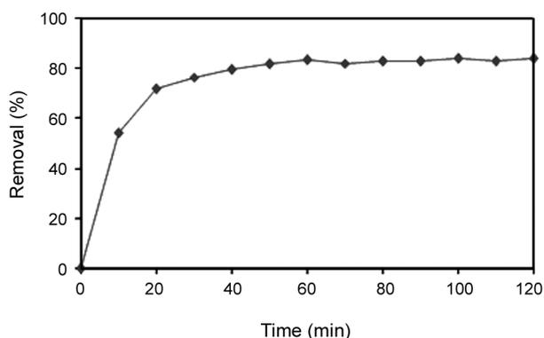
**Figure 1:** Effect of contact time on adsorption of CNB onto MWCNTs.  $[CNB]_0=16$  mg/L;  $[MWCNTs]_0=0.1$  g/250mL; pH=5.4.
