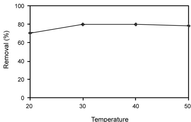
**Figure 5:** Effect of temperature on adsorption of CNB onto MWCNTs. [CNB]<sub>0</sub>=16 mg/L; [MWCNTs]<sub>0</sub>=0.1 g/250mL, [pH]<sub>0</sub>=5.4; Contact Time=60 min.
