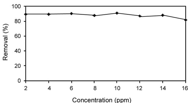
**Figure 4:** Effect of CNB concentrations on adsorption of it onto MWCNTs. [MWCNTs]<sub>0</sub>=0.1 g/250mL, [pH]<sub>0</sub>=5.4; Contact Time=60 min.
