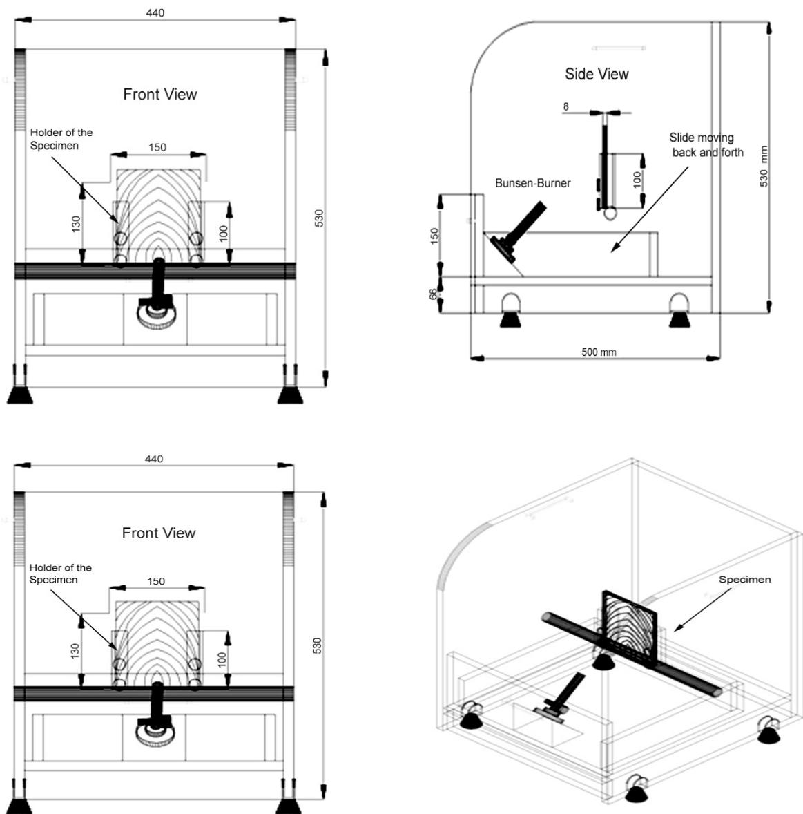
**Figure 1:** Schematic picture of the slide fire testing apparatus (SFTA) (invented by the second author under Iranian Patent No. 67232; approved by Iranian Research Organization for Science and Technology under license No. 3407).
