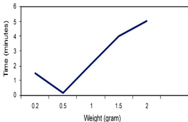
**Figure 16:** Optimization of support weight in 2g catalyst.
