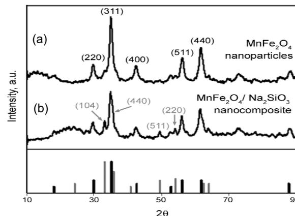
Figure 3: XRD of MnFe<sub>2</sub>O<sub>4</sub> (a: pure b: in the presence of sodium metasilicate).
