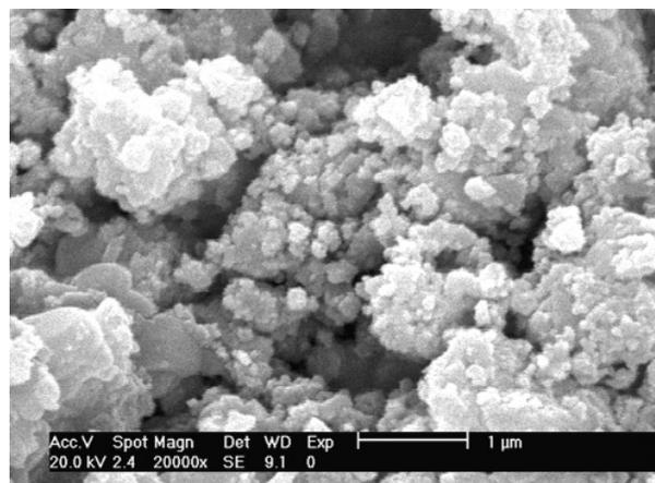
**Figure 9:** SEM of nanocomposite with zeolite support.
