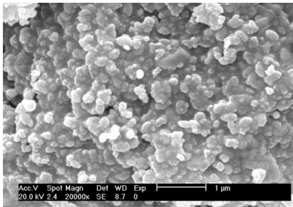
**Figure 7:** SEM of nanocomposite with sodium metasilicate support.
