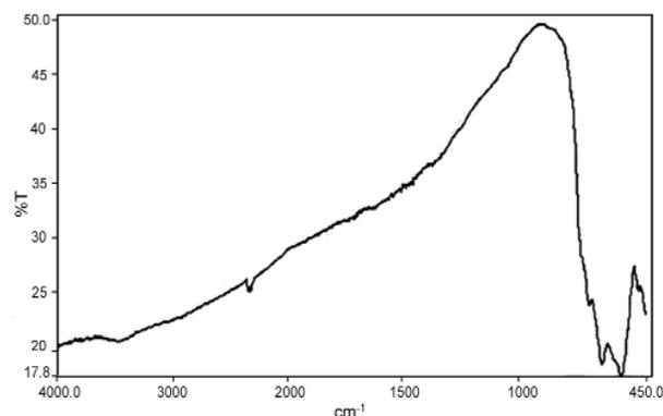
Figure 2: IR spectrum of MnFe<sub>2</sub>O<sub>4</sub>
