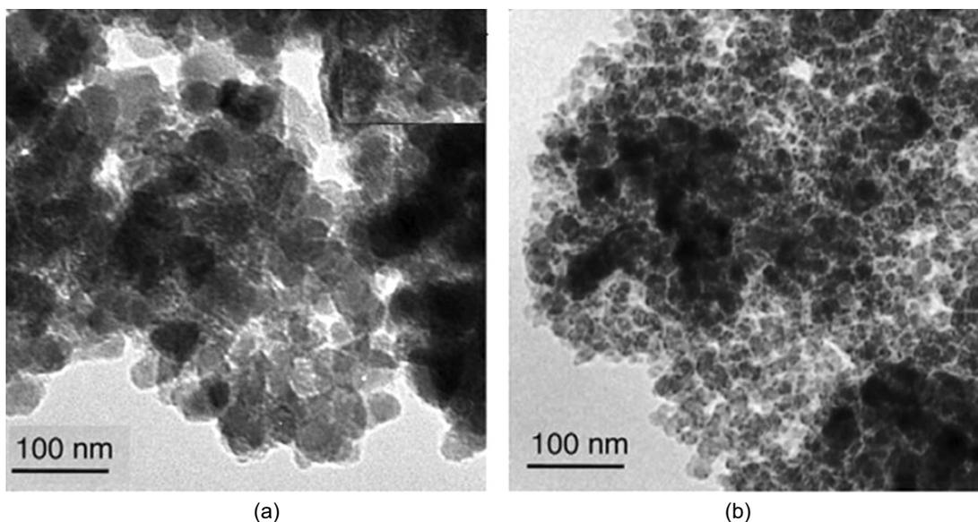
**Figure 13:** TEM image of the iron-manganese oxide nanoparticles (a: pure b: in the presence of sodium metasilicate).
