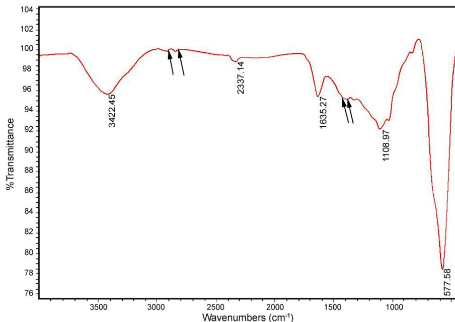
**Figure 3:** FTIR spectrum of un-calcined  $\text{CoFe}_2\text{O}_4$  nano-particles.
