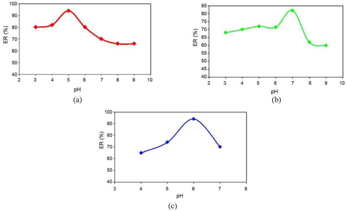
**Figure 7:** Effect of pH on a) SDS coating step, b) PDTCAA modification step, and c) the extraction efficiency of  $10 \mu\text{g L}^{-1}$  Pb(II) ions using the proposed MSPE procedure.
