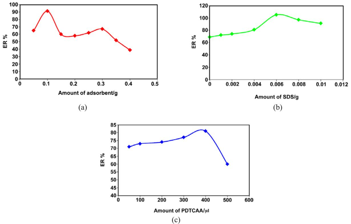
**Figure 8:** Effect of amount of a) SDS-PDTCAA- $\text{Fe}_3\text{O}_4$  NPs, b) SDS and c) PDTCAA on the adsorption characteristics of  $10 \mu\text{g L}^{-1}$  Pb(II) ions using the proposed MSPE procedure.
