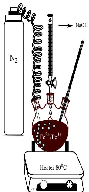
**Figure 1:** The schematic of the synthesis process of  $Fe_3O_4$  NPs.
