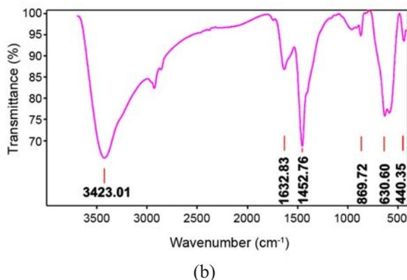
**Figure 5:** FTIR spectra of a)  $\text{Fe}_3\text{O}_4$  NPs, and b) SDS-PDTCAA- $\text{Fe}_3\text{O}_4$  NPs.
