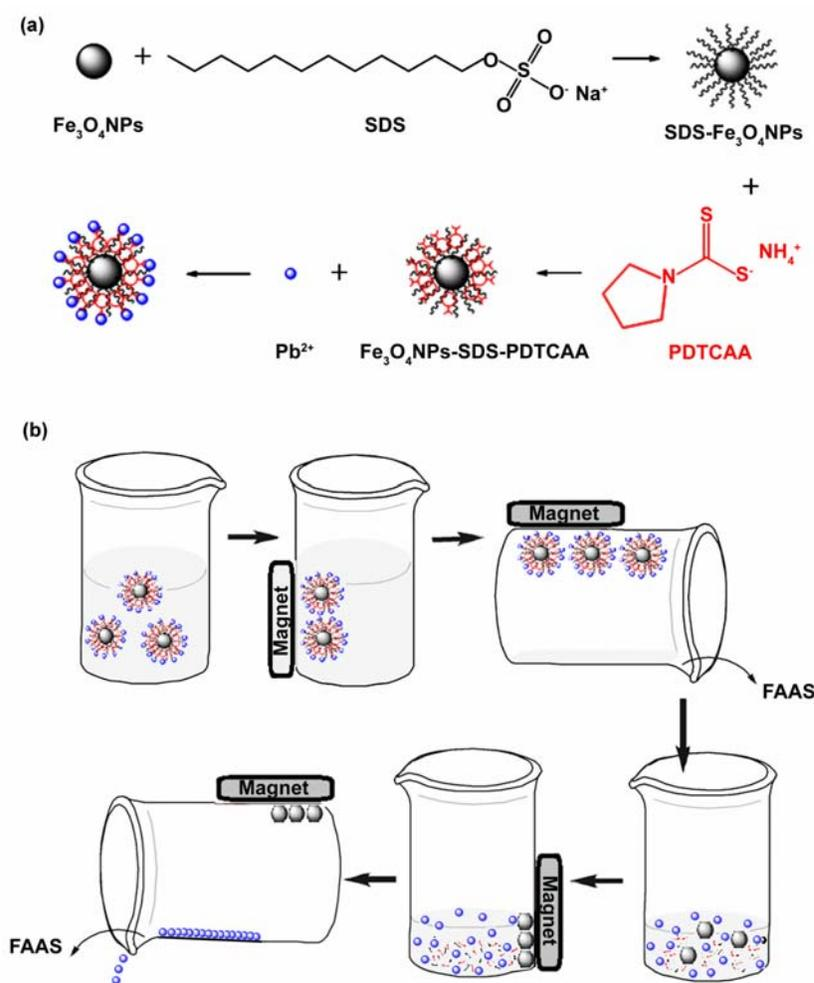
**Figure 2:** a) Schematic illustration of the modification of  $\text{Fe}_3\text{O}_4$  NPs with SDS and PDTCAA groups and adsorption of Pb(II) ions, b) application of SDS-PDTCAA- $\text{Fe}_3\text{O}_4$  NPs for separation and preconcentration of Pb(II) ions in water samples based on MSPE.
