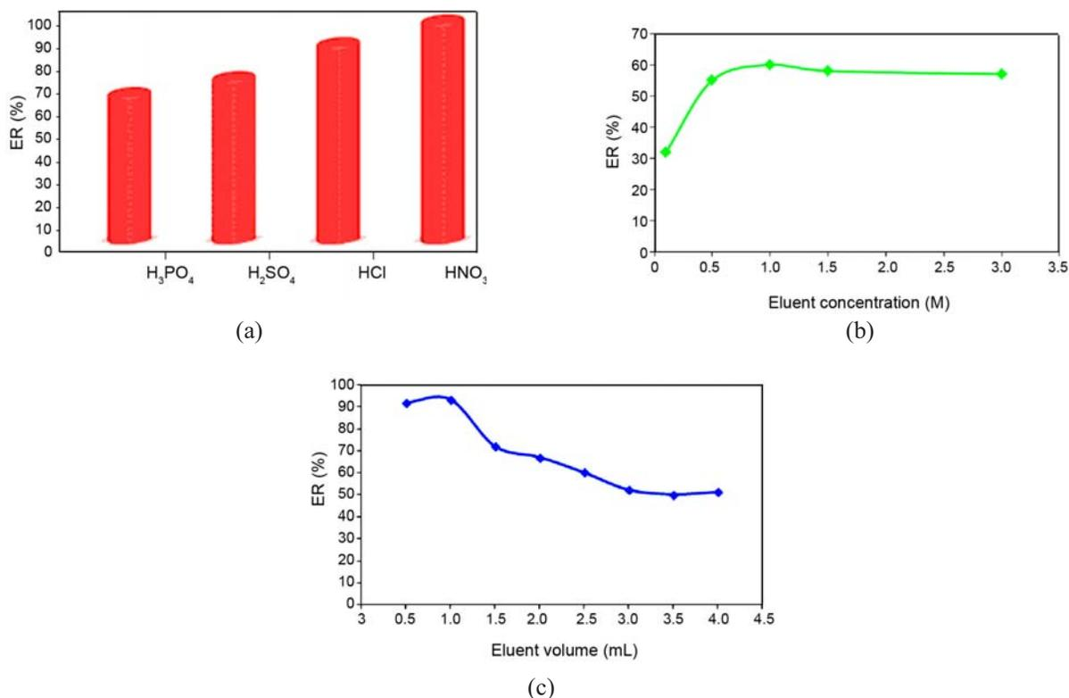
**Figure 9:** Effect of a) type, b) concentration, and c) volume of eluent (HNO<sub>3</sub>) on the desorption characteristics of 10 µg L<sup>-1</sup> Pb(II) ions from SDS-PDTCAA-Fe<sub>3</sub>O<sub>4</sub> NPs using the proposed MSPE procedure.
