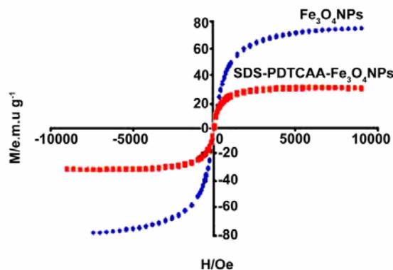
**Figure 6:** The magnetic behavior of a)  $\text{Fe}_3\text{O}_4$  NPs, and b) SDS-PDTCAA- $\text{Fe}_3\text{O}_4$  NPs.
