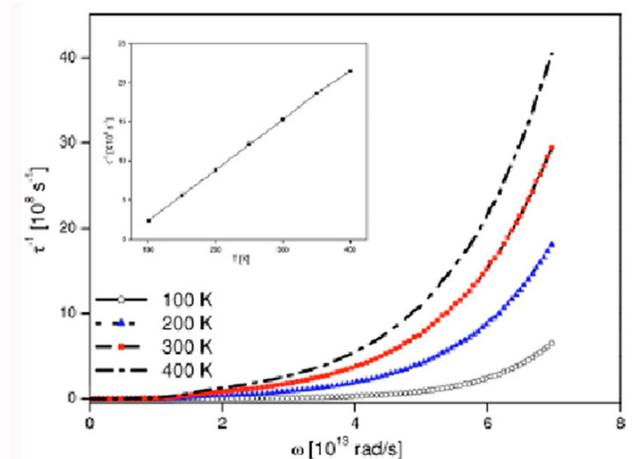
Fig. 2: Relaxation rates of Umklapp process of (6, 0) SW-CNT.
