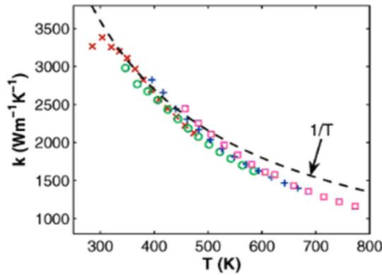
Fig. 4: Thermal conductivity of SWCNT in the temperature range 300-800K.
