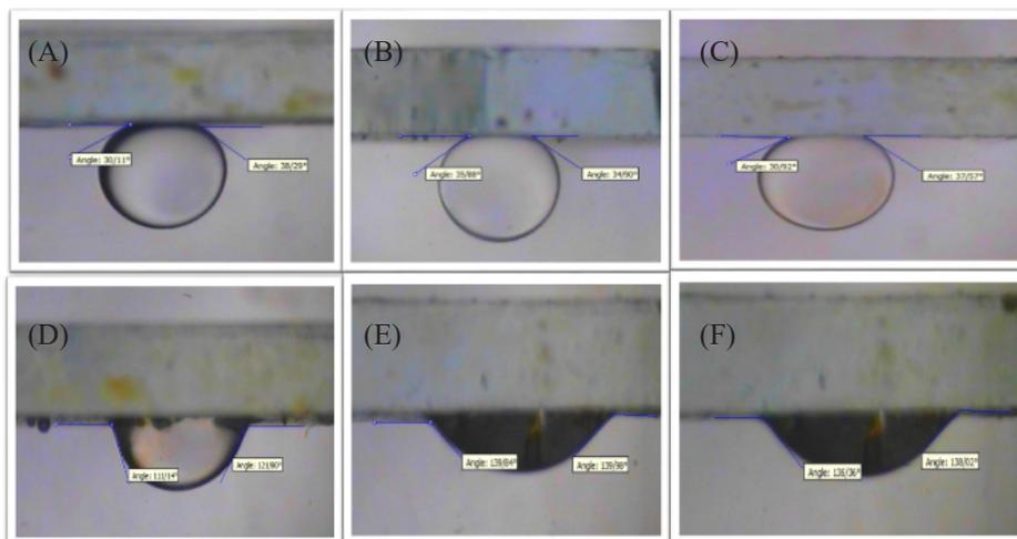
Fig. 5. A - 0.01% salinity at 80 degree temperature , B - 0.05% salinity at 80 degree temperature , C - 0.1% salinity at 80 degree temperature , D - 0.2% salinity at 80 degree temperature , E - 0.2% salinity at 80 degree temperature , F - 1% salinity at 80 degree temperature
