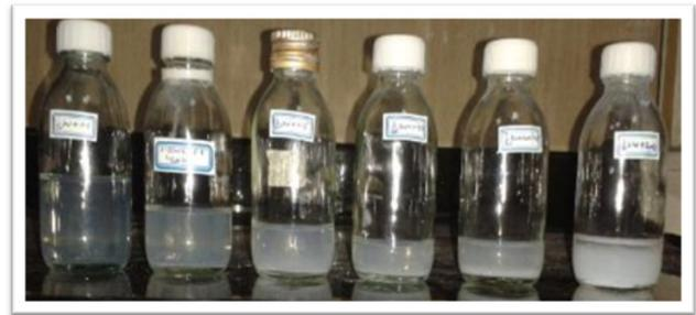
Fig. 2. Nanoparticles combinations with different concentrations in 20 times diluted seawater
