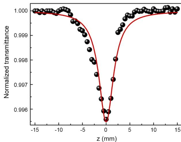
Fig. 4. The normalized transmittance and theoretical simulation curves (solid lines) as a function of sample position in the open aperture Z-scan configuration for ZrO<sub>2</sub>/TiO<sub>2</sub>/ZnO nanocomposites.
