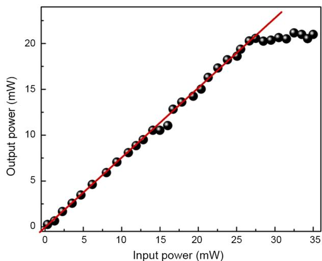
Fig. 3. Output power versus input power plot of  $ZrO_2/TiO_2/ZnO$  nanocomposites prepared by the sol-gel method.
