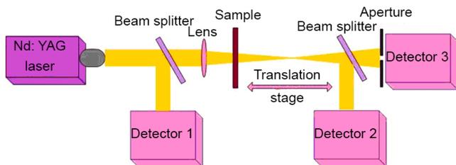
Fig. 1. The experimental setup for the measurement of the nonlinear optical parameters in  $ZrO_2/TiO_2/ZnO$  nanocomposites synthesized by the sol-gel method.
