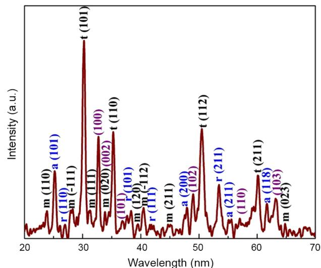
Fig. 2. XRD pattern of  $ZrO_2/TiO_2/ZnO$  nanocomposites. The diffraction peaks marked in black indicate monoclinic (m) and tetragonal (t) phases of  $ZrO_2$ . The diffraction peaks marked in purple and blue represent the wurtzite-type hexagonal crystalline structure of ZnO and anatase (a) and rutile (r) phases of  $TiO_2$ , respectively.
