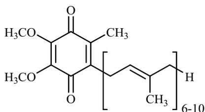
Figure 1: The chemical structure of coenzyme Q10
