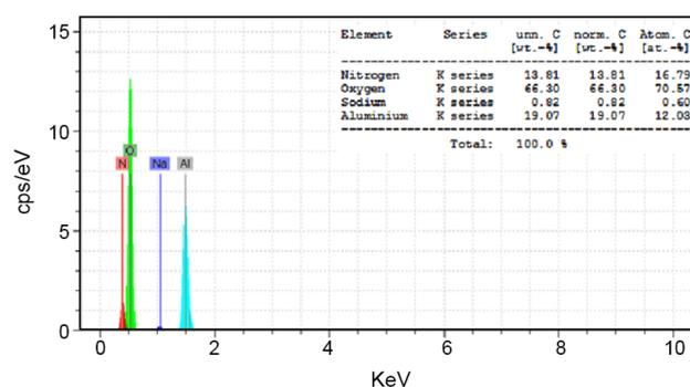
Fig. 4. EDS spectra of the as-synthesized Al<sub>2</sub>O<sub>3</sub>.
