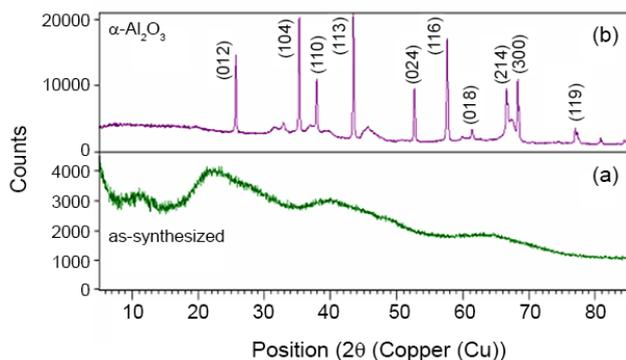
Fig. 1. XRD pattern of Al<sub>2</sub>O<sub>3</sub> nanocrystals, (a) as-synthesized and (b) annealed at 1000°C
