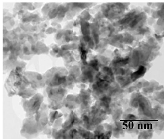
Fig. 3. TEM image of the as-prepared Al<sub>2</sub>O<sub>3</sub> nanoparticles
