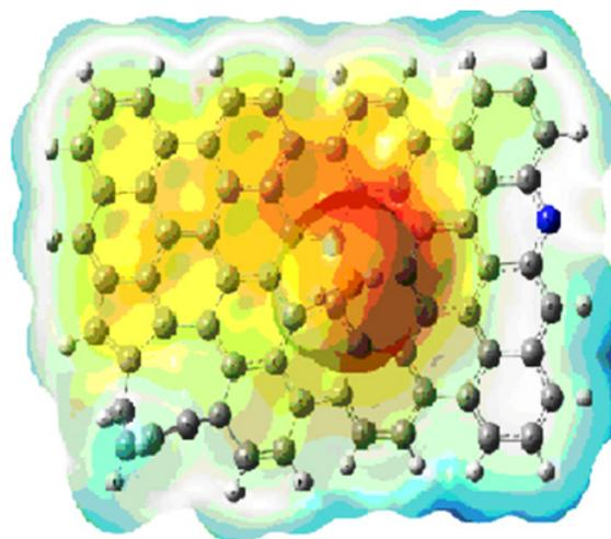
Fig. 3. The molecular electrostatic potential (MEP) of the nitrogen-doped graphene sheet and  $H_2S$ .
