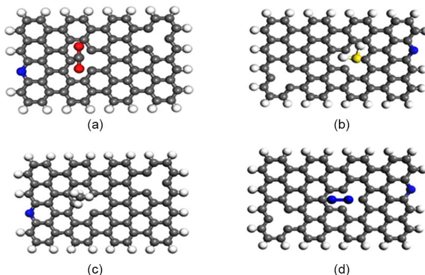
Fig. 1. Geometries of a) CO<sub>2</sub>, b) H<sub>2</sub>S, c) CH<sub>4</sub> and d) N<sub>2</sub> adsorbed on nitrogen-doped graphene sheet.
